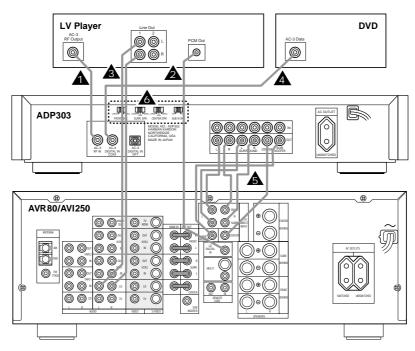
Use this setup for connection to an AVR80, AVI250 or other compatible products equipped with 6 Channel Direct inputs.
