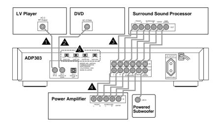
Use this setup for connection to an external surround sound processor or preamplifier.
