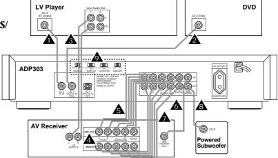
Although AV receivers that have both preout/main-in jacks for all five surround channels as well as a subwoofer output were not designed for Dolby Digital applications, you may use them with the ADP303 by using the following steps:
